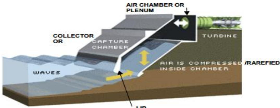
**Figure 1.** The diagram of OWC (House, 2013)
