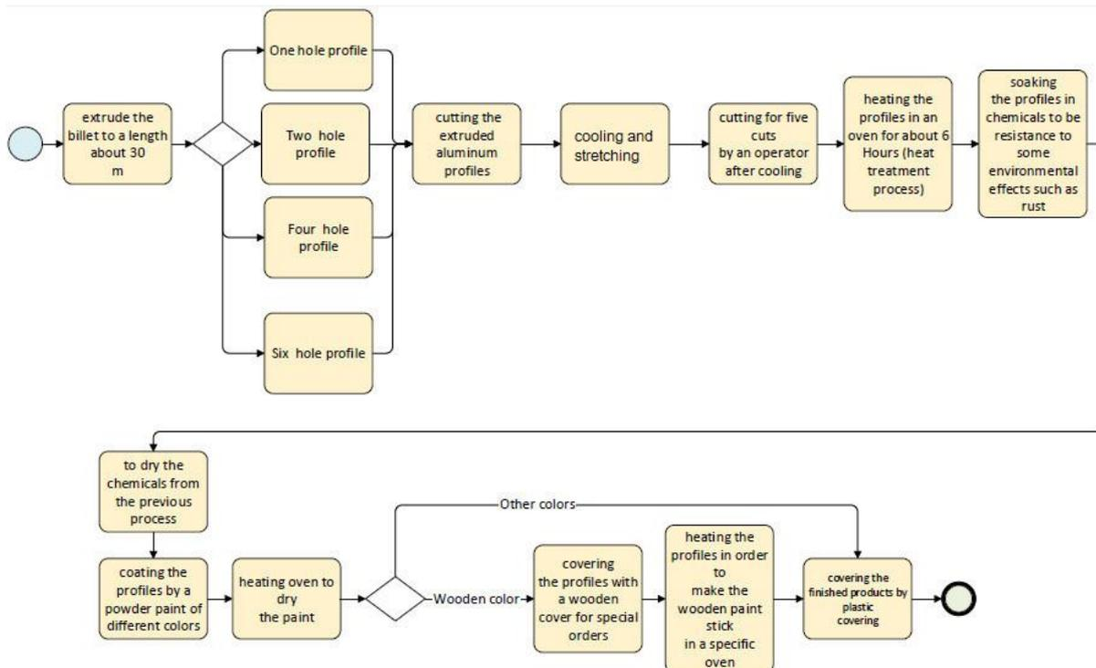
Figure 1: Flow chart of Aluminum Extrusion Plant
