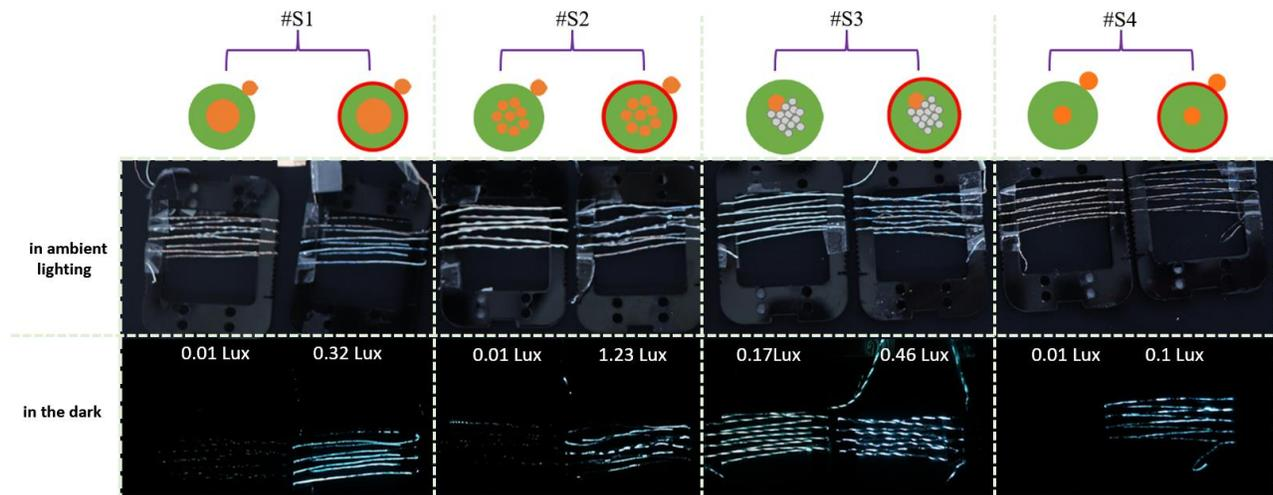
**Figure 3:** *EL Response of The Different EL Fibers with And Without PEDOT: PSS (Red Region) Measured in The Dark and In Ambient Lighting (Illuminance  $\pm 0.01$  Lux).*
