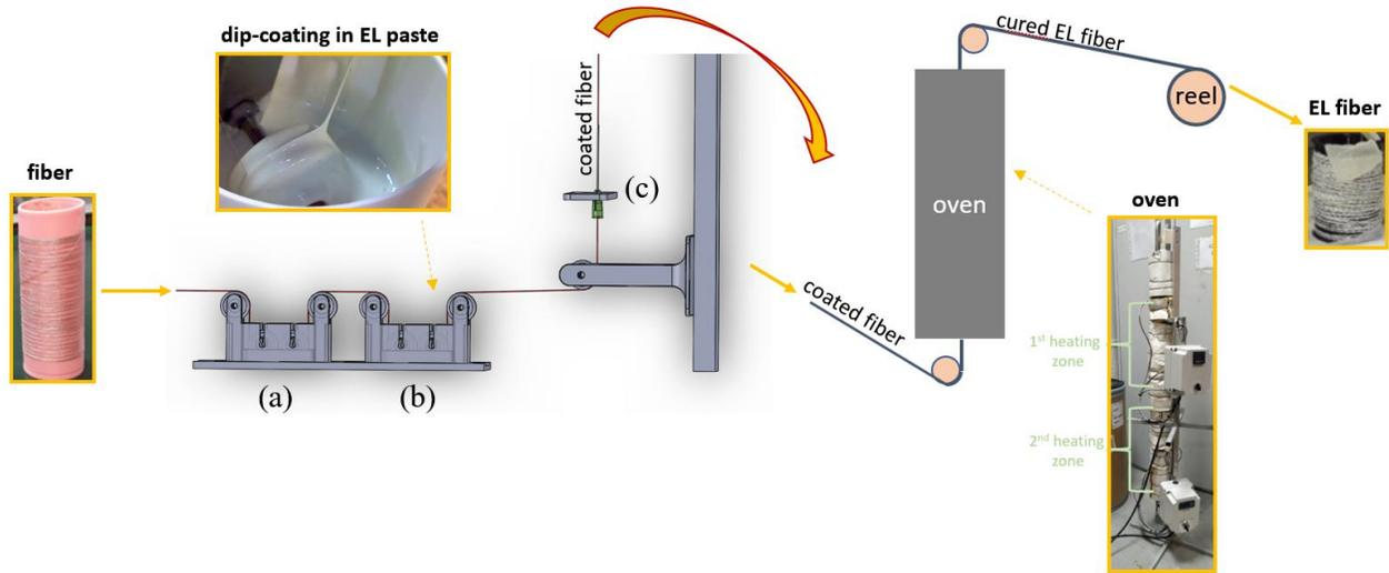
**Figure 1:** Setup developed for the fabrication of the EL fibres: dip-coating, curing, and reeling systems.
