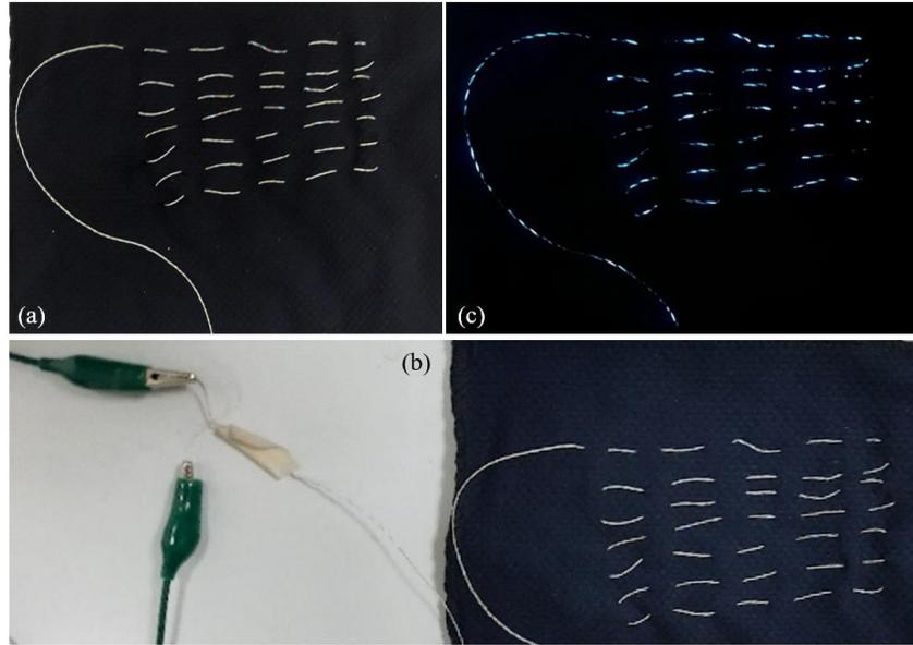
**Figure 5:** *EL Fibers Manual Integration in Textiles*
