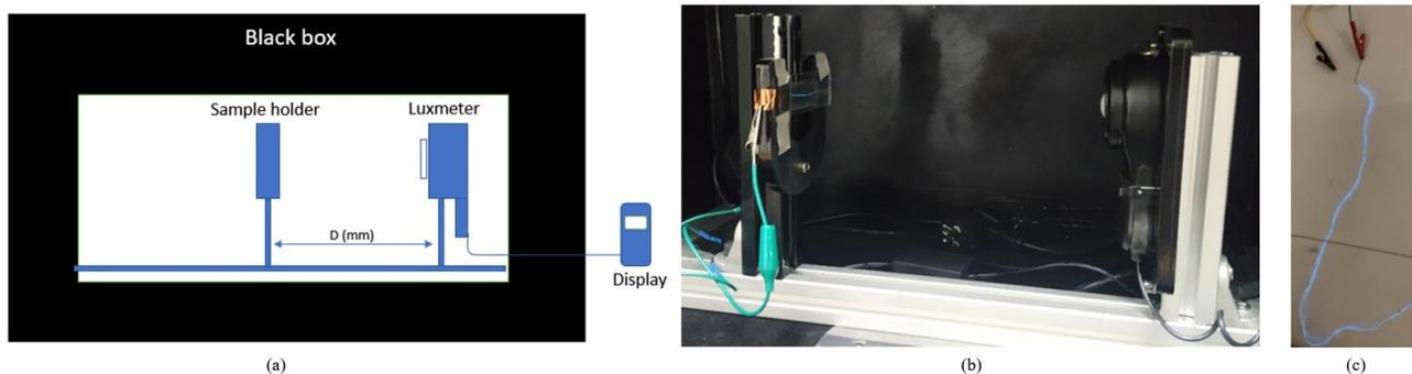
**Figure 2:** Schematics (a) and photography (b) of the setup for illuminance measurements.
