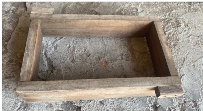
Figure 1: Wooden mold measuring 5.5 x 14 x 25.5 cm
