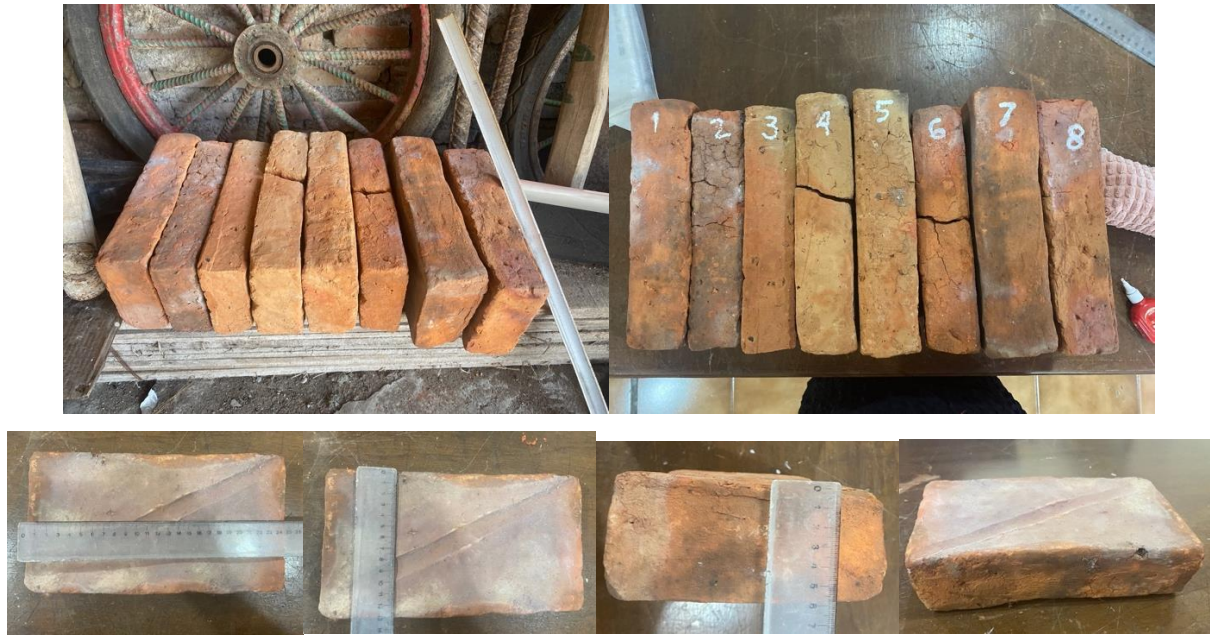
Figure 2: Repair bricks Production Results
