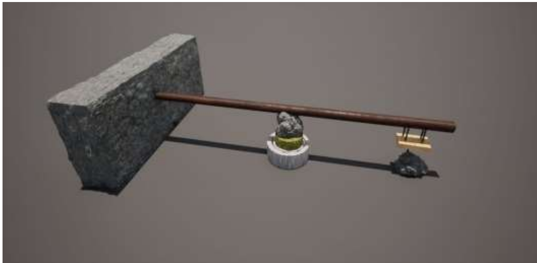
Figure 13: 3D reconstruction of the olive press in its resting state. Final pressing stag. Axonometric view
